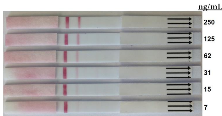
Figure 1: Serial dilutions of Mouse IgG Subclass Standard.
