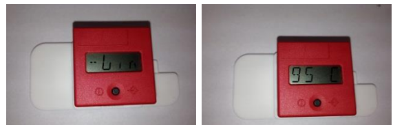
Figure 5 - Once programmed with the included RFID card, press the button a third time to read the cassette
